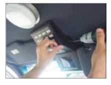
View of control head being mounted with wires already attached to connections
